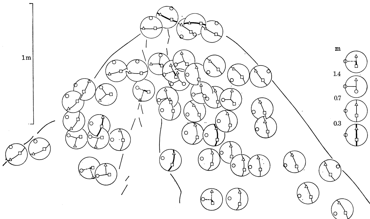
FIGURE 3. The magnetic fabric of a fold in greywacke (Moseley 1968, fold I). The principal susceptibility directions (maximum, \square ; intermediate, \triangle ; minimum, \circ ) are plotted as equal area stereograms projected on to the plane of section.
